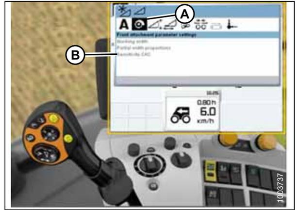
Figure 5.233: CLAAS Combine Display, Console, and Joystick Lever
