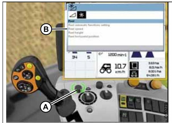
Figure 5.236: CLAAS Combine Display, Console, and Joystick
