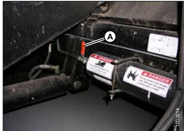
**Figure 5.76: Combine Accumulator ON/OFF Switch**
