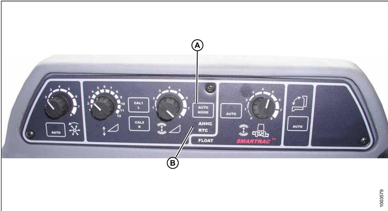
1. Press AUTO MODE (A) button until AHHC LED light (B) begins flashing. If RTC light is flashing, press AUTO MODE (A) button again until it switches to AHHC.
