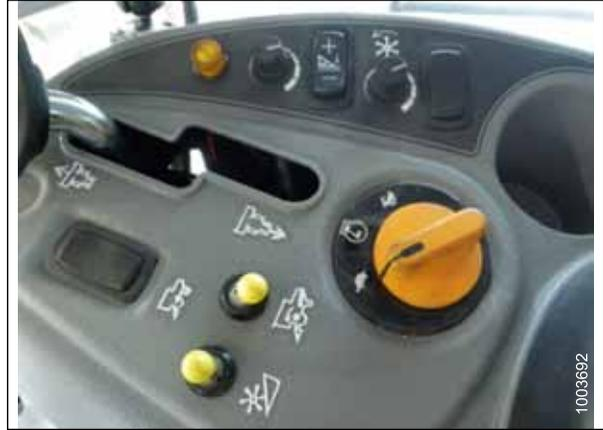
**Figure 5.58: Height Adjustment Knob on Combine Control Console**
