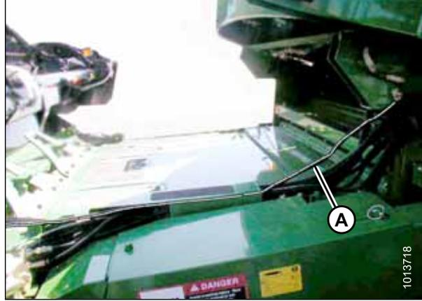
Figure 3.69: 60/70 Series Harness Routing
