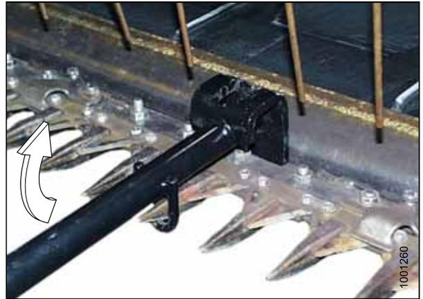
Figure 6.8: Guard Tips – Upward Adjustment
