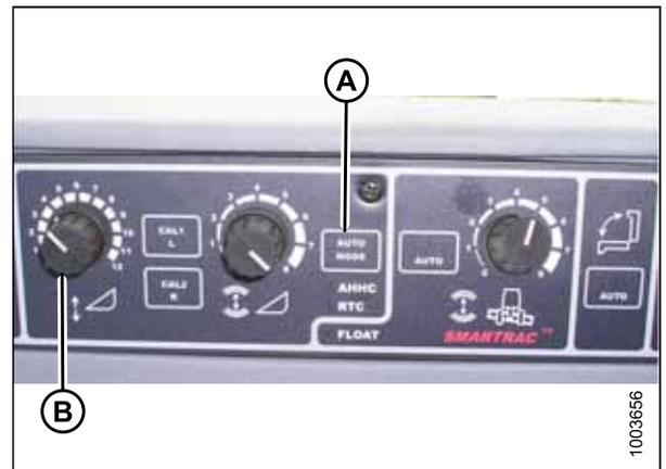
Figure 5.78: Auto Header Height Control Console
