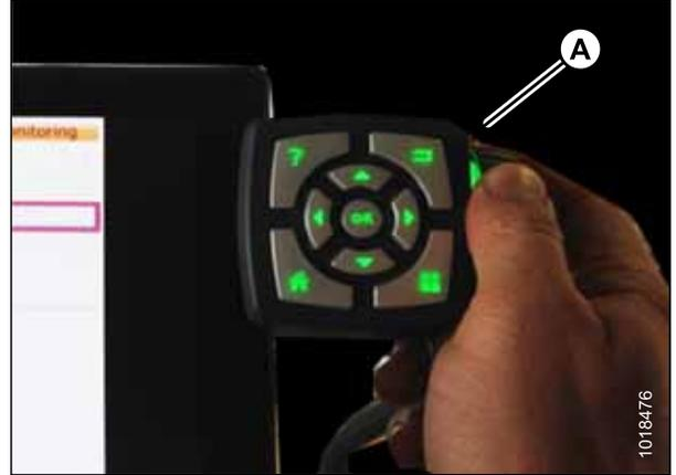
Figure 5.115: Scroll Wheel for Adjustments
