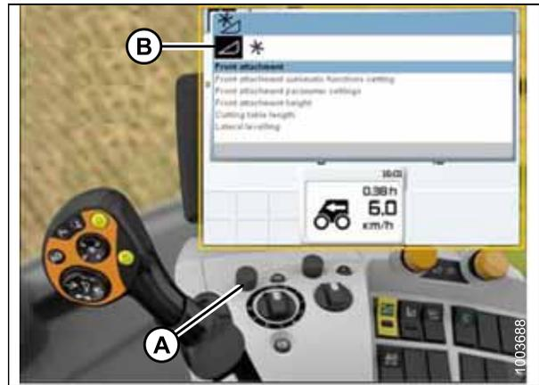
Figure 5.225: CLAAS Combine Display, Console, and Joystick
