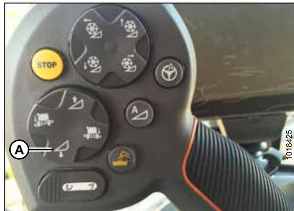
Figure 5.104: Header Down Switch
