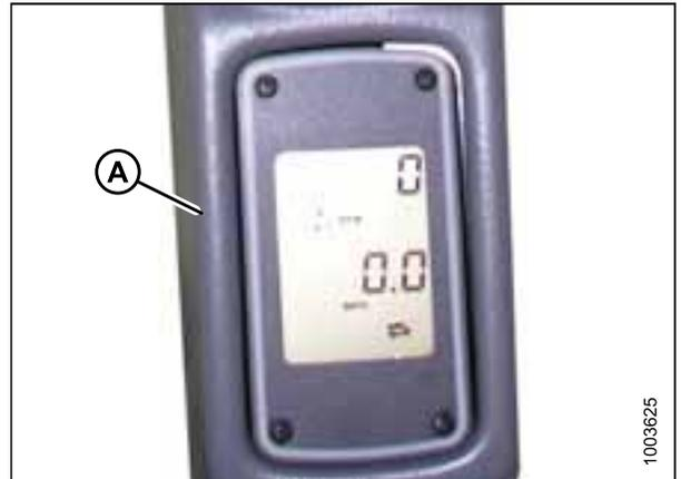
**Figure 5.81: Tachometer**
