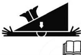
**Rest header on ground or engage mechanical locks before going under unit. See Operators Manual.**
