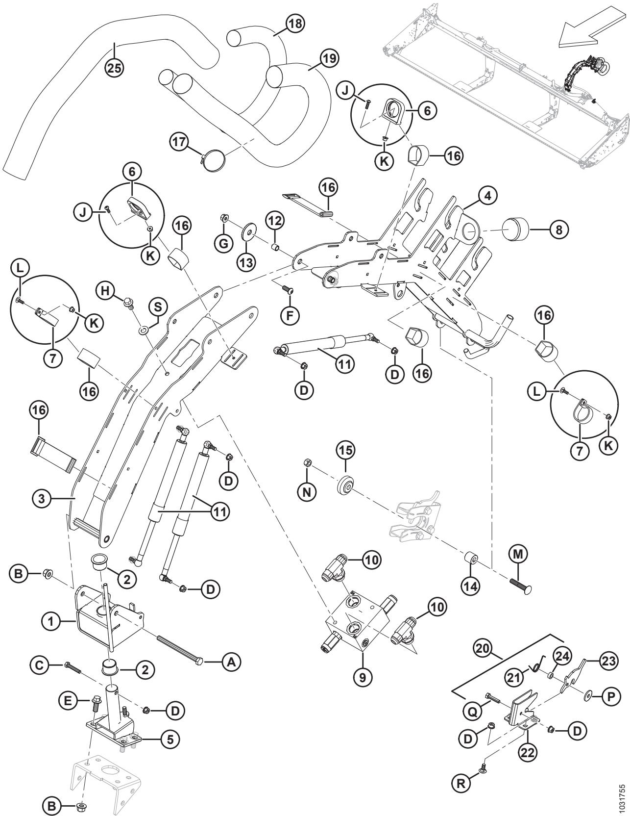
**M1 SERIES WINDROWER HYDRAULIC COMPLETION – SUPPORT ARM AND LATCH**
