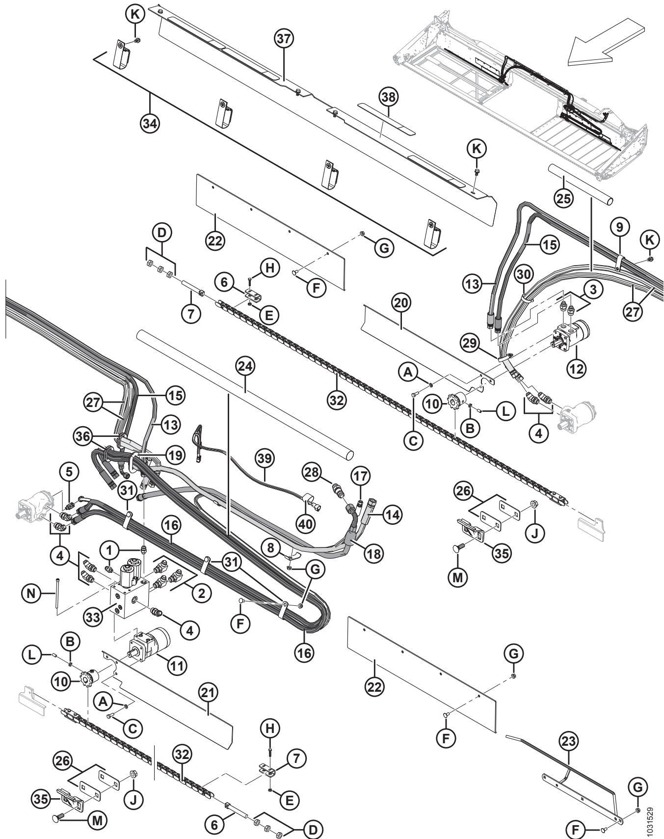
**DRAPE DRIVE – HYDRAULIC DECK SHIFT, D125X (2019 AND PRIOR)**
