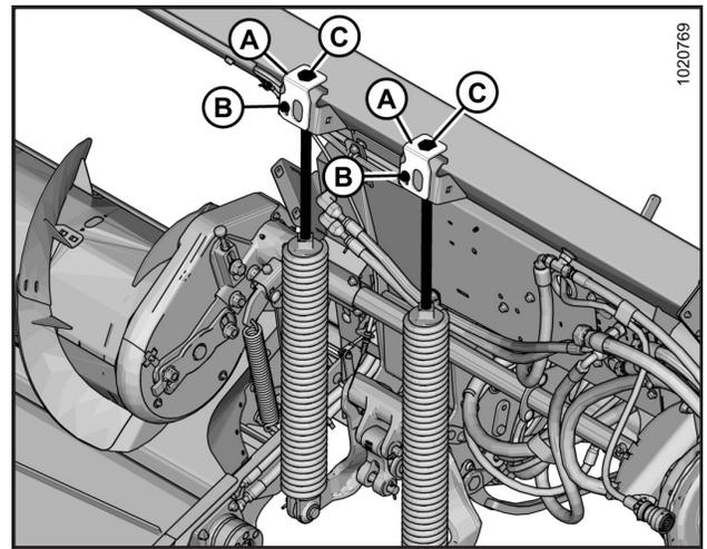
Figure 5: Float Adjustment Bolts – Left Side
