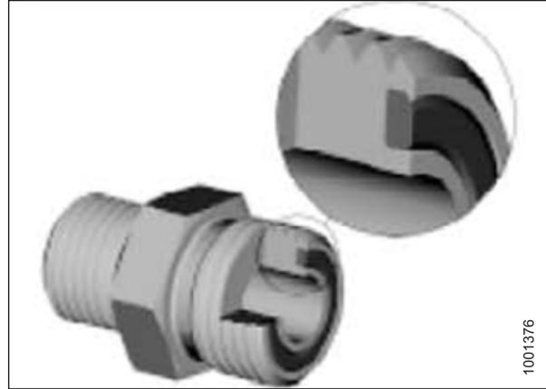
Figure 6.13: Hydraulic Fitting
