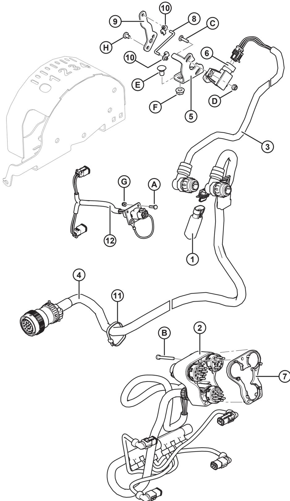
**CLAAS LEXION SÉRIE 500/700 – KIT DE ACOPLAMENTO ELÉTRICO**
