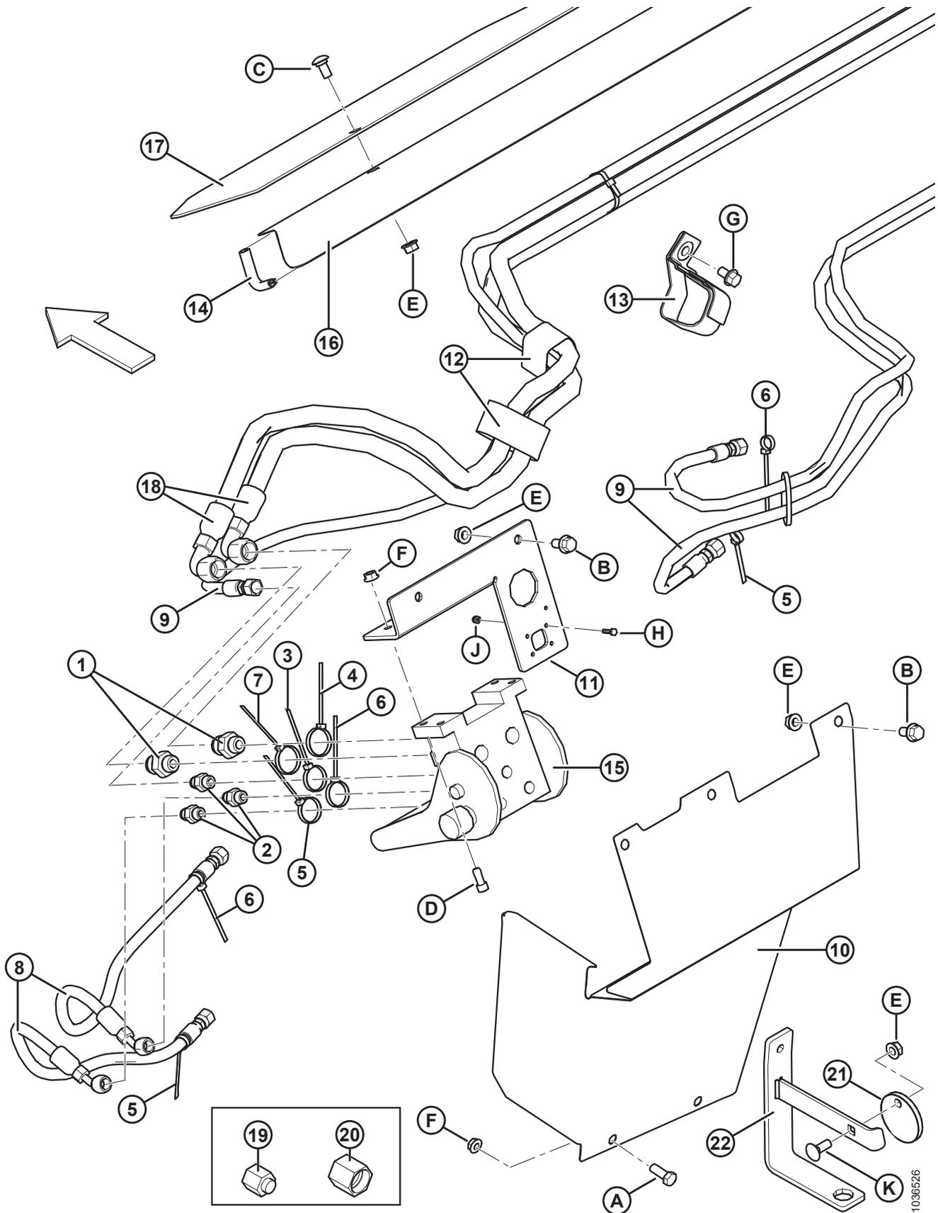
**CASE IH E NEW HOLLAND CR/CX – KIT DE ACOPLAMENTO HIDRÁULICO**
