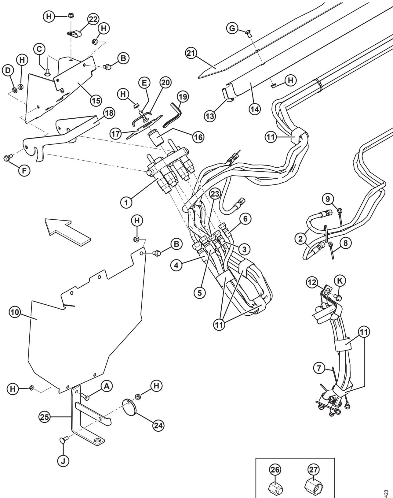
**KIT DE ACOPLAMENTO HIDRÁULICO – JOHN DEERE SÉRIE 60/70/S, 2016 E ANTERIORES**
