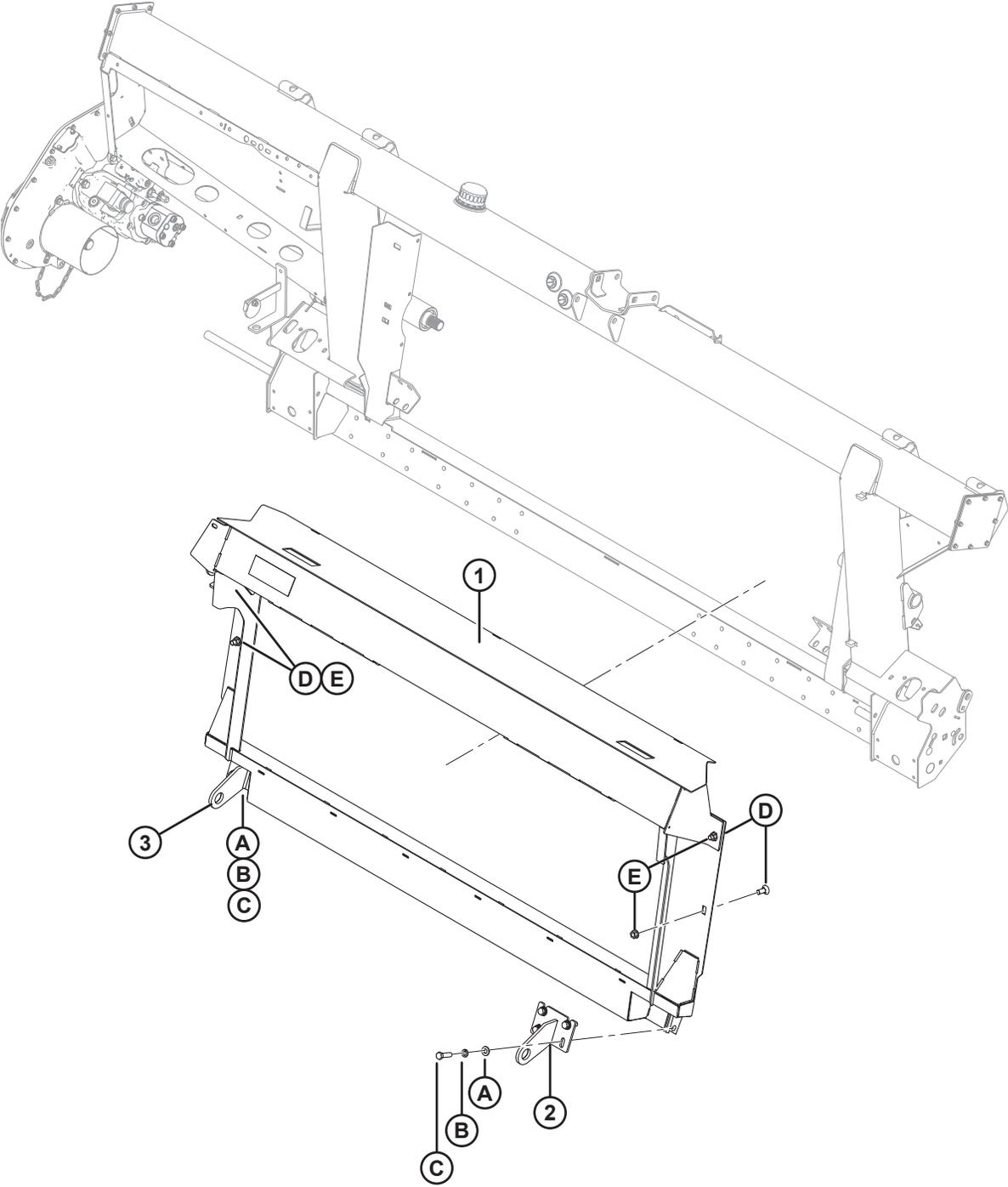
**KIT DE ACOPLAMENTO DO ADAPTADOR – JOHN DEERE SÉRIES 50/60/70/S**
