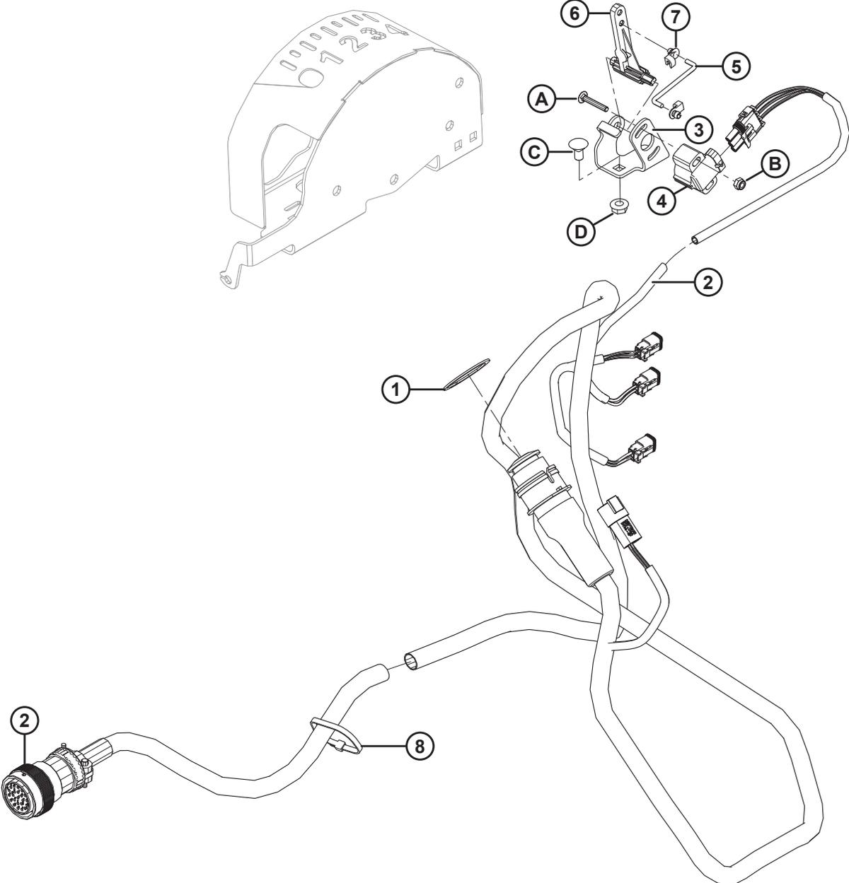
**KIT DE ACOPLAMENTO ELÉTRICO – JOHN DEERE SÉRIES 50/60/70/S**
