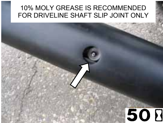
DRIVE-LINE SLIP JOINT
