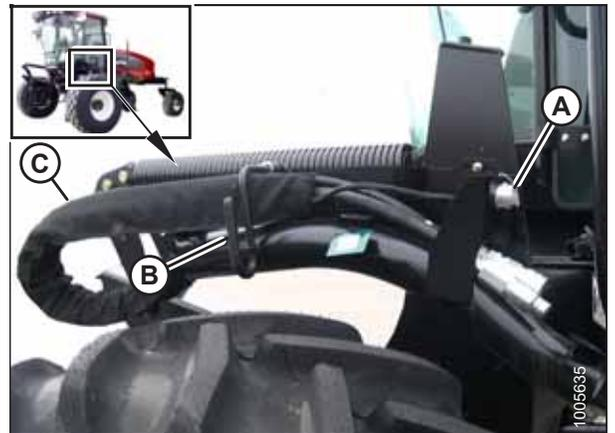
Figure 3.30: Support Bracket and Hose Bundle
