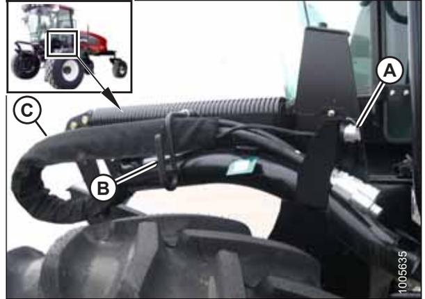
Figure 3.59: Support Bracket and Hose Bundle
