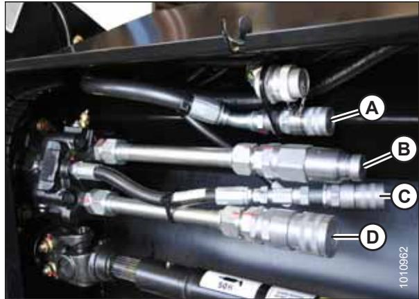
Figure 3.62: A40D Hose Connections – 5.4 m (18 ft.) Header Shown
