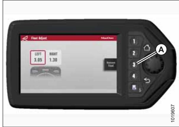
Figure 3.122: HPT Display – Adjusting Float
