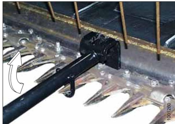
Figure 4.28: Guard Tip – Upward Adjustment
