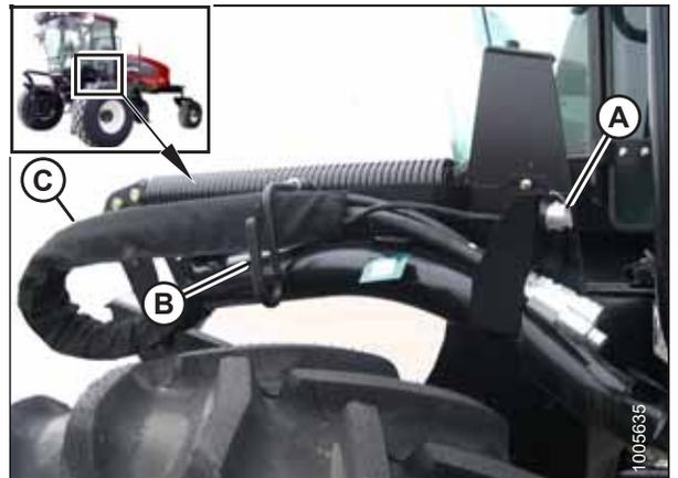
Figure 3.16: Support Bracket and Hose Bundle
