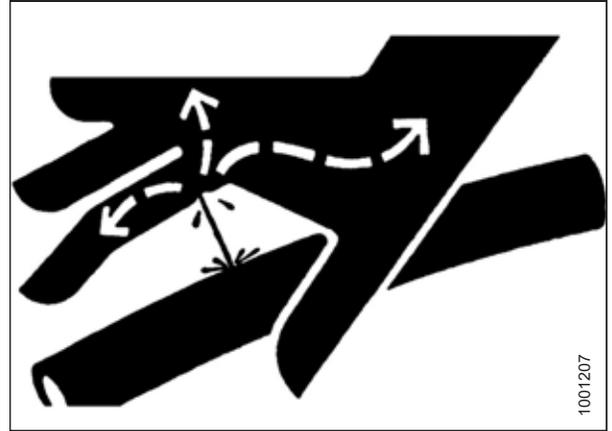
Figure 4.14: Hydraulic Pressure Hazard
