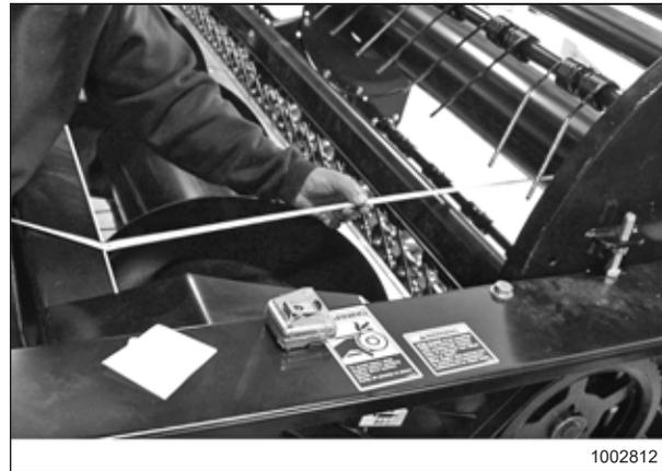
Figure 3.100: Measuring Reel Fore-Aft Offset
