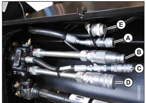
Figure 3.91: A40D Hose Connections – 5.4 m (18 ft.) Header Shown
