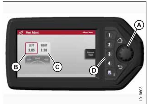
Figure 3.120: HPT Left and Right Float Settings
