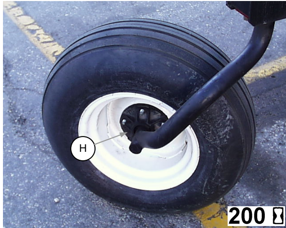
CASTER WHEEL HUB BEARINGS (H) TWO FITTINGS
