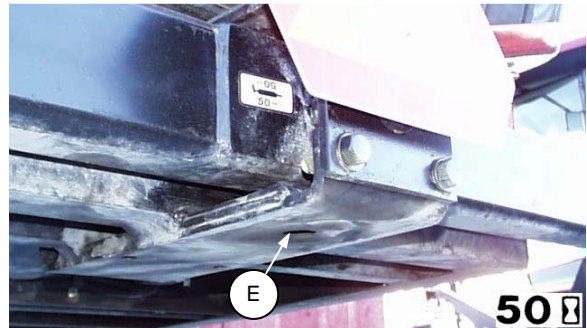
WALKING BEAM PIVOT (E) - ONE FITTING
