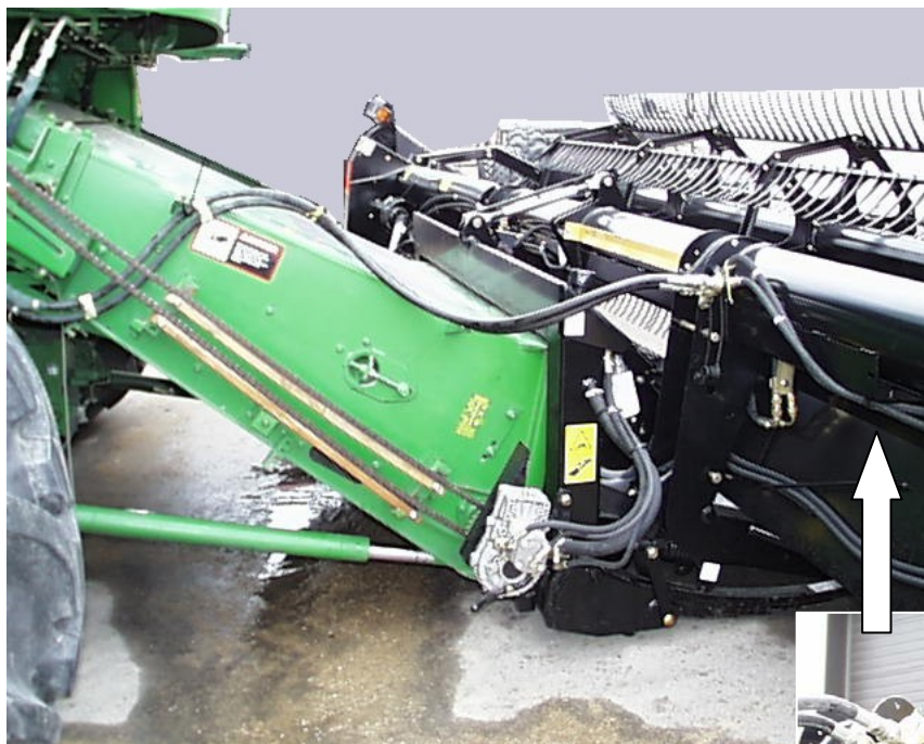
PUMP MOUNTING – PRIOR TO 50 SERIES & COMBINE TO HEADER CONNECTIONS, R/H SIDE
