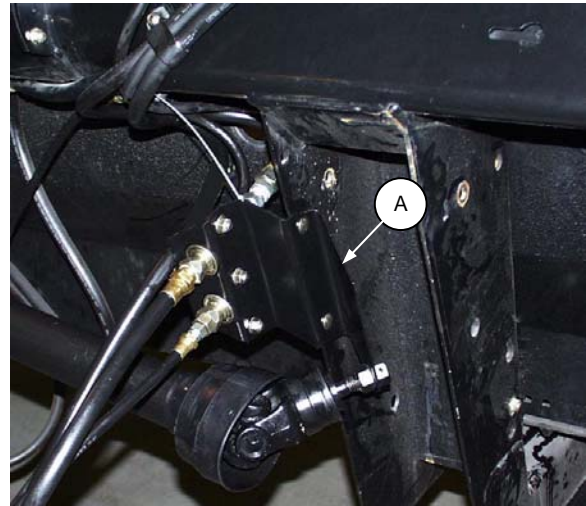
ATTACH REEL DRIVE MOUNTING PLATE TO HEADER L/H LEG
