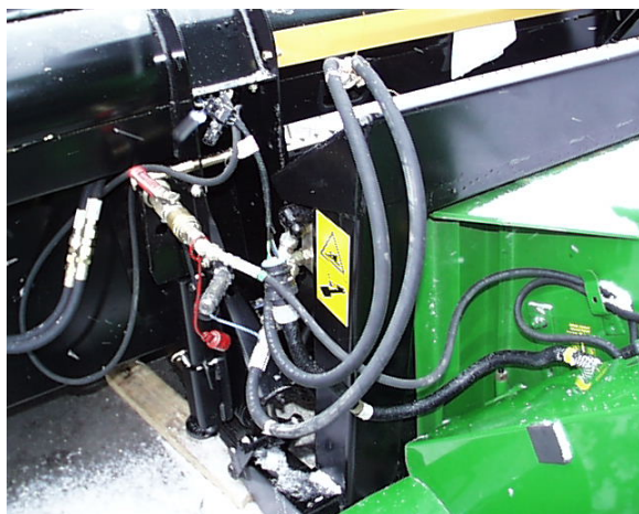
COMBINE TO HEADER CONNECTIONS - LEFT SIDE
