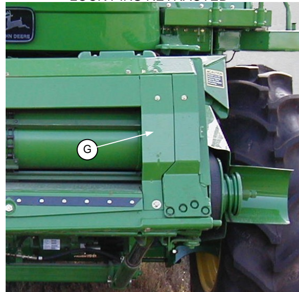
REMOVE CONTOUR MASTER COMBINE FILLER PLATES
