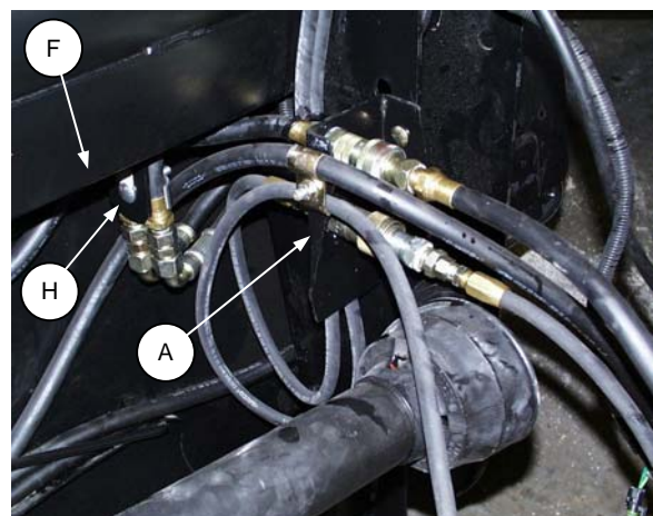
ATTACH REEL DRIVE MOUNTING PLATE TO HEADER L/H LEG
