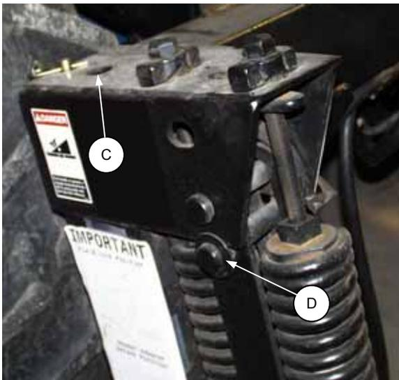
R/H FLOAT LOCK-OUT PIN - ENGAGED
