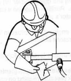
CHECK PROPERLY FOR LEAKS
