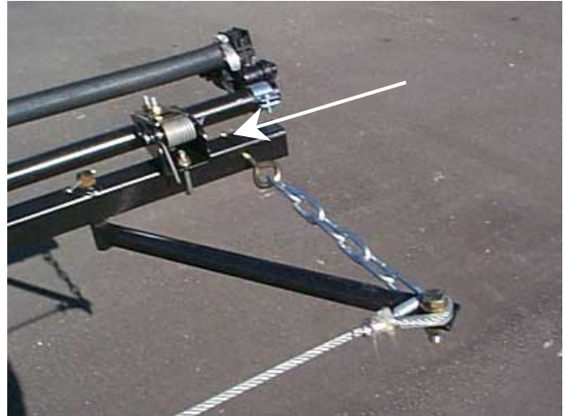
Adjust draw bolt to change wire cable tension.
