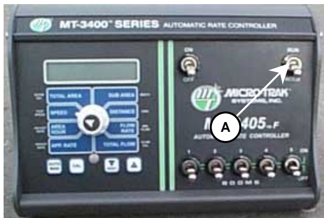
Boom activation switches on the MT-3405 automatic rate controller.
