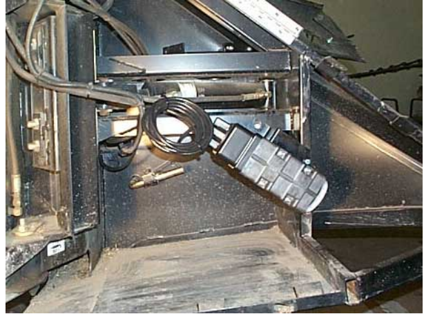
Location of the DICKEY-john Radar velocity sensor
