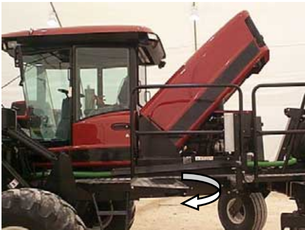
Engine Access Panel Open
