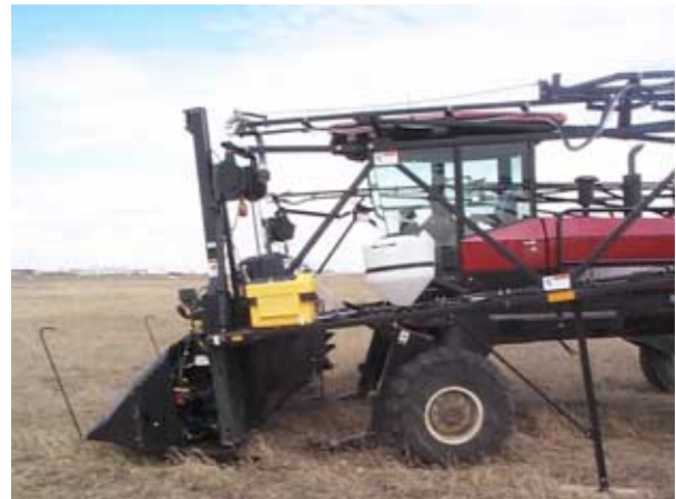
Line up the lift linkage with the sprayer attachment legs and slowly drive the tractor forward.
