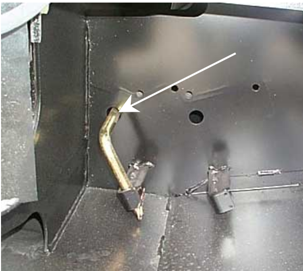
Pin located through the bottom hole in the lift linkage on each side of the main frame.
