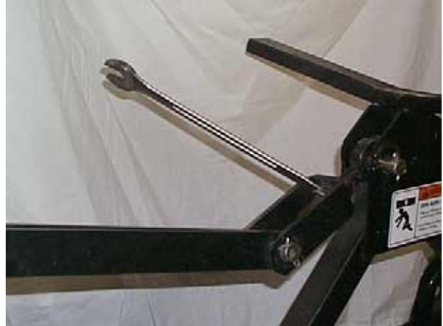
Tighten the draw bolt at link to the Vertical Suspension to level the boom.
