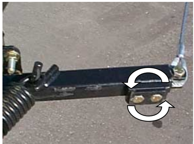
Latch plate on break away boom tip.
