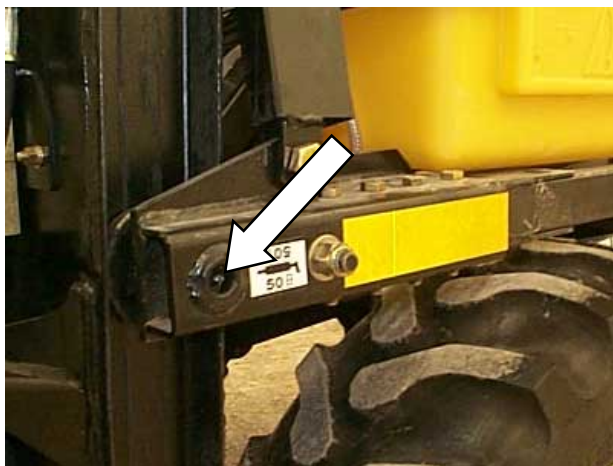
Bottom trolley wheel spindles (2 Grease Points on each side). Grease when booms are in FIELD position.
