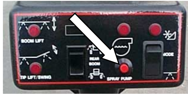
Depress switch on the pedestal in the cab to engage pump.
