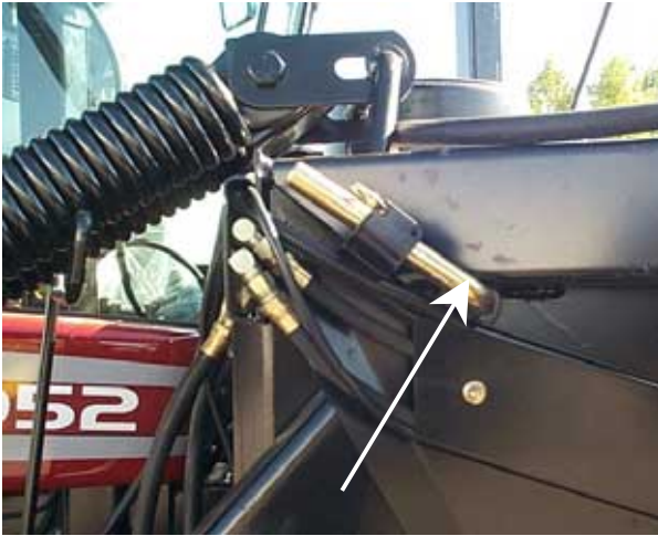
Pin located through the top hole in the lift linkage on each side of the main frame.
