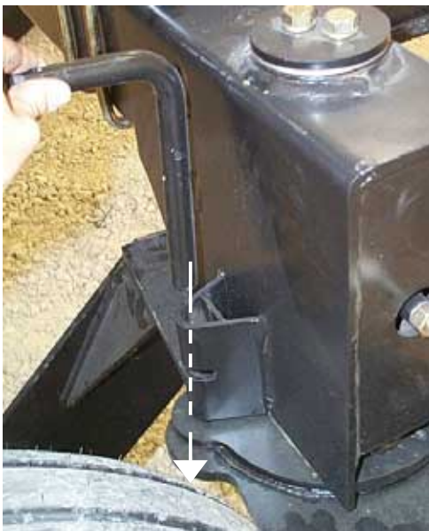
Secure the rear caster wheel prior to transporting the sprayer on a trailer.
