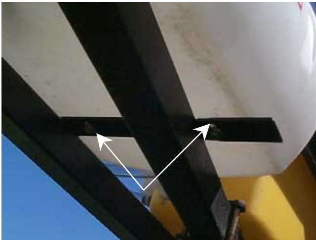
Secure with bolts underneath the tank.
