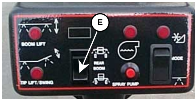
Rear center boom height control switch.
