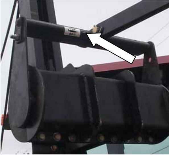
Vertical suspension (1 Grease point on each side)
