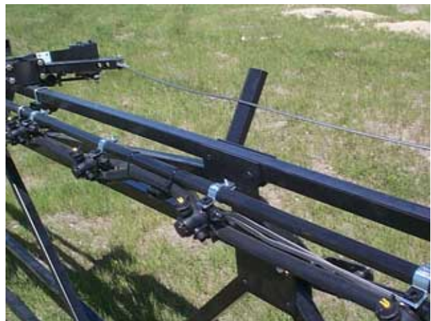
Adjust boom tip to land at the center of the cradle.
