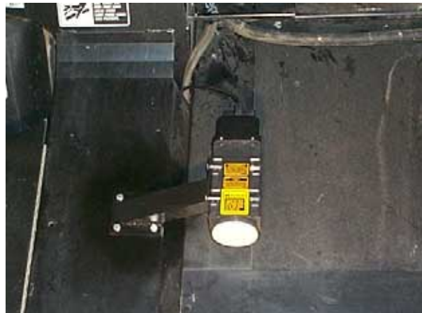
Radar can be mounted in front of the tank for higher crop applications.
