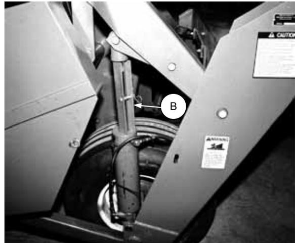
LIFT CYLINDER STOPS - ENGAGED
