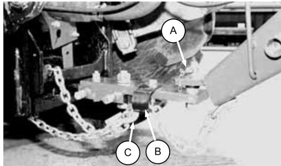
SECURE HITCH PIN AND CHAIN
