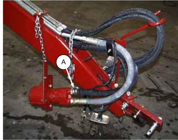
DRAIN RESERVOIR AT PUMP SUPPLY HOSE
