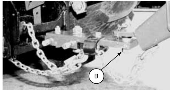
**CHECK HITCH PIN LOCK NUT**
