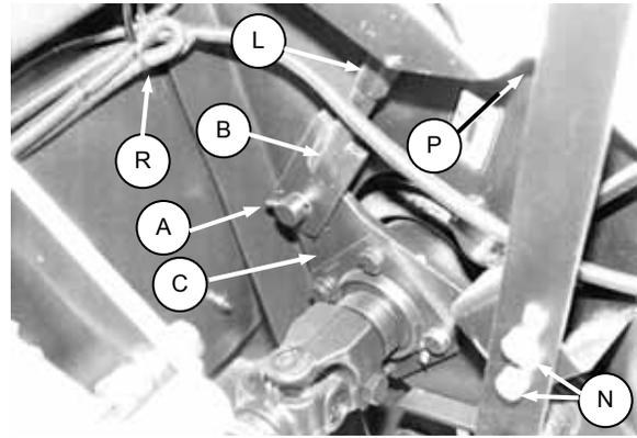
REMOVE ROLL GAP ADJUSTMENT ROD
