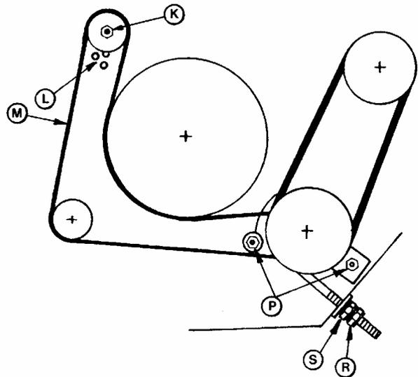
AUGER DRIVE CHAIN AND BELT TENSION ADJUSTMENT
