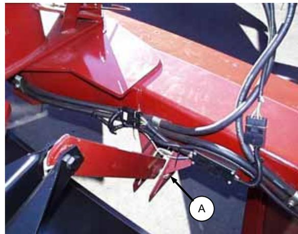
ADJUST LINK TO CENTER OF SLOT
