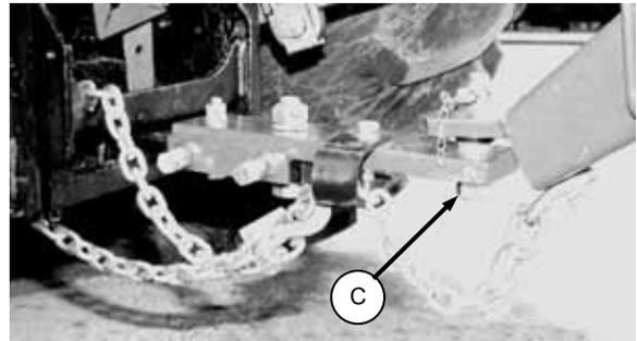
CHECK HITCH PIN LOCK NUT
