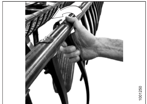
Figure 4.6: Removing Plastic Finger
