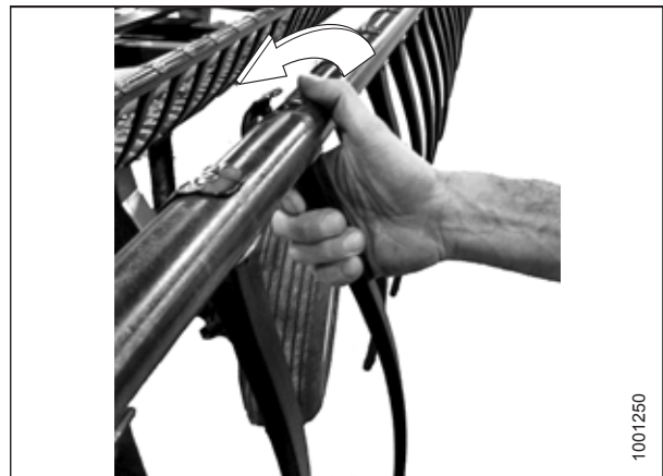
Figure 4.15: Removing Plastic Finger
