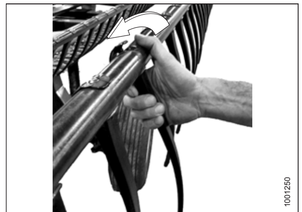
Figure 4.19: Removing Plastic Finger
