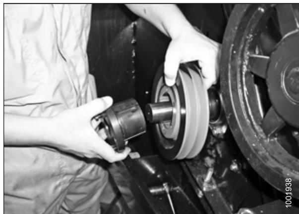
Figure 3.25: Hub and Pulley Reinstallation
