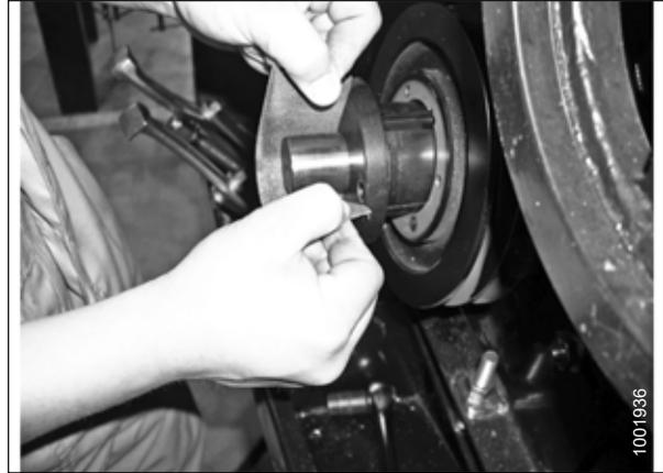
Figure 3.23: Shaft Cleaning
