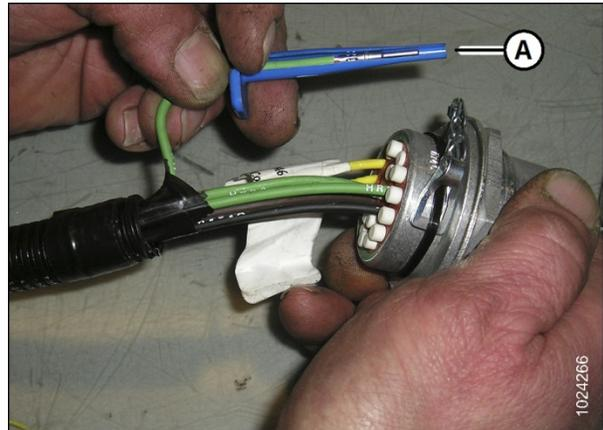
**Figure 7: Wire Removed**
