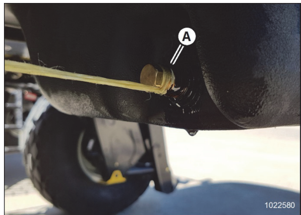
Figure 5: O-Ring and Sealant on Fitting
