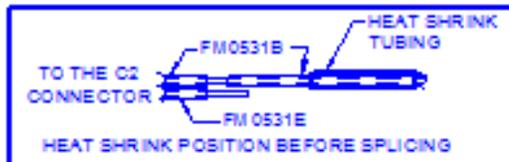
8. To make the new splice, wrap the end of the exposed FM0531E wire around the exposed section of the FM0531B wire then complete the connection by soldering the wires together using the rosin core solder.
