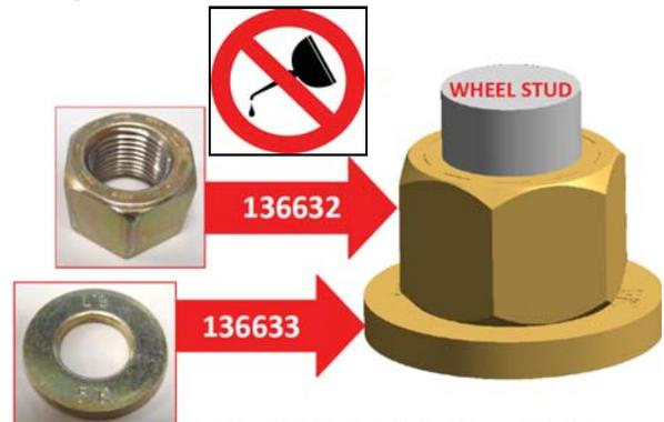
Nut should be installed dry. Do not lubricate threads with oil or products such as Never Seez®
