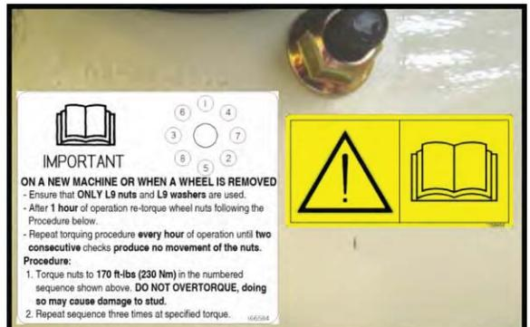
Figure 5 – New Drive Wheel Decal MD #166584 And READ MANUAL Decal MD #166454
