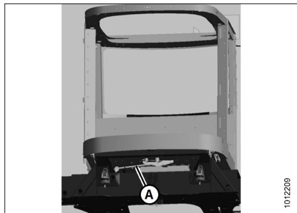
Figure 10: Front View of Cab with Lateral Link Below
