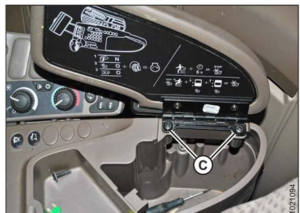
Figure 3.13: Installing Control Panel
