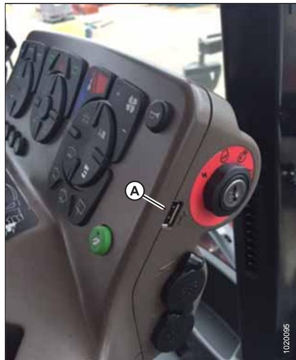
Figure 3.13: USB Port on Console
