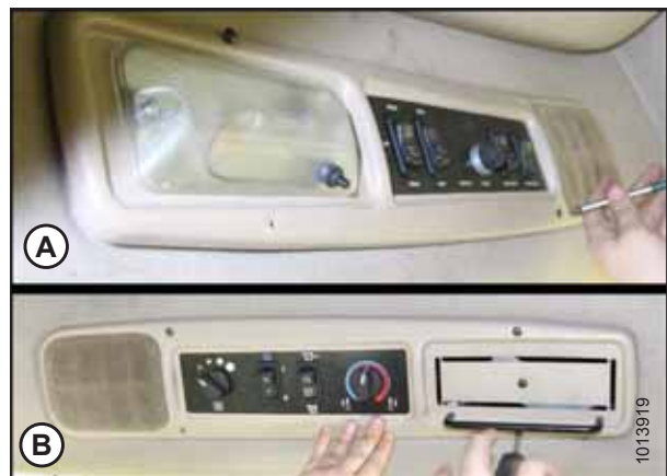
Figure 3.5: Headliner Switch Panels
