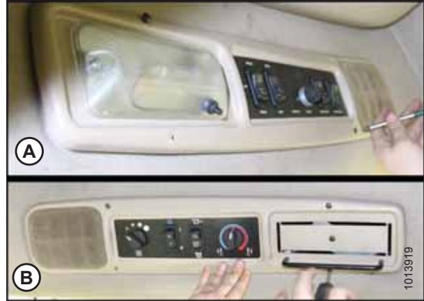
Figure 3.15: Headliner Switch Panels
