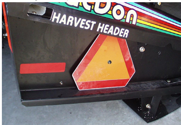
INSTALL SMV SIGN (SINGLE SICKLE DRIVE HEADERS)
