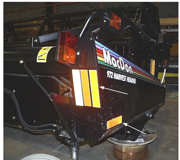
RIGHT END – TWO REFLECTORS DOUBLE SICKLE HEADER
