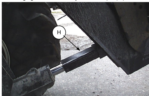
ENGAGE LIFT CYLINDER STOPS
