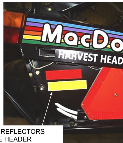
RIGHT END – TWO REFLECTORS DOUBLE SICKLE HEADER
