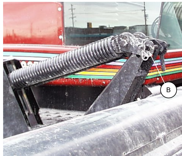
ATTACH FLOAT SPRINGS
