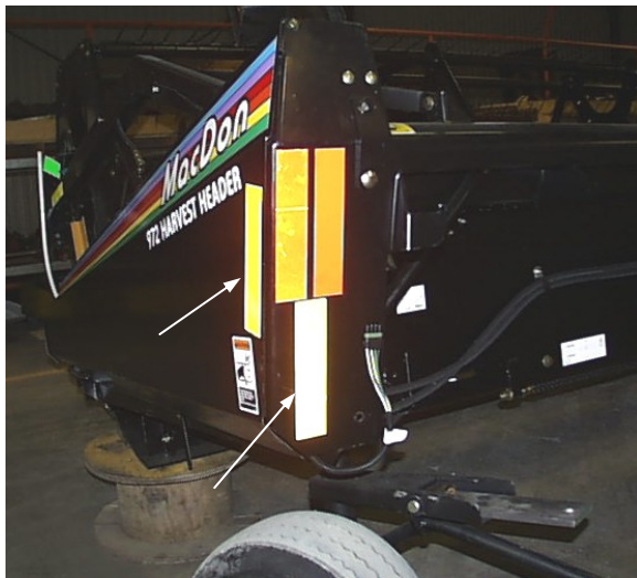
LEFT END – TWO REFLECTORS
