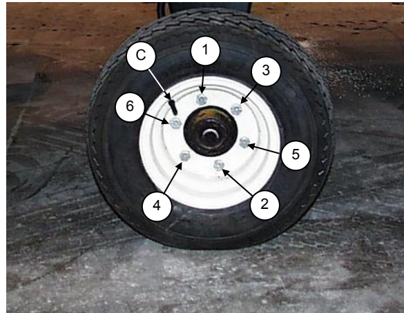
BOLT TIGHTENING SEQUENCE
