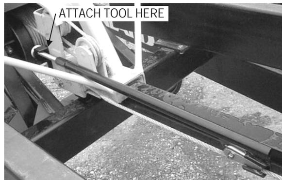
INSTALL CABLE WITH CABLE INSTALLATION TOOL
