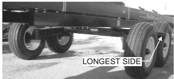
BOLT AXLE BEAM TO FRAME
