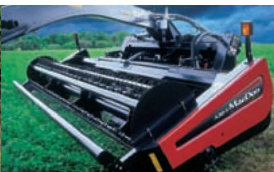
A30 Pull-Type Mower Conditioner Sizes: 14' (4.3 m) and 16' (4.9 m)
