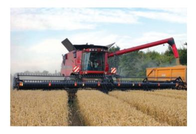
"I had seen them working elsewhere, and was particularly impressed by the positive feed, and the lighter overall weight from the lack of an auger, and the wider range of header adjustment, all of which I hoped would give us more output from the combine than with a standard header.
